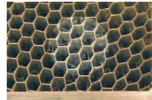
Schlegel's standard honeycomb vent uses 2 layers of 1/8" cell X 1/4" thick laid at 90°, this is known as cross cell. Cross cell honeycomb improves shielding performance by eliminating any polarizing effects.
