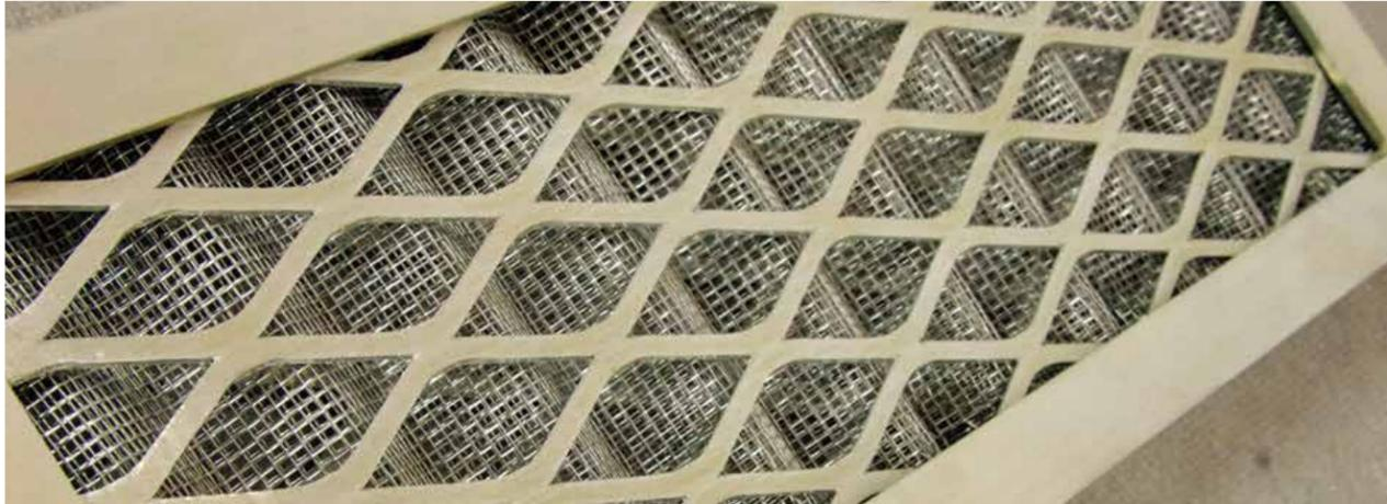
Aluminum EMC & dust filter ventilation panel consist of 3 layers of pleated aluminum woven mesh trapped between an expanded aluminum kick-plate then held in a rigid extruded aluminum mounting frame, The 3 layers of pleated wire mesh are separated by the pleats being of different height enabling the vent to have a high dust holding capacity. The vent panel can be used dry or air filter oil can be applied to the aluminum filter media to assist in dirt and dust retention.
