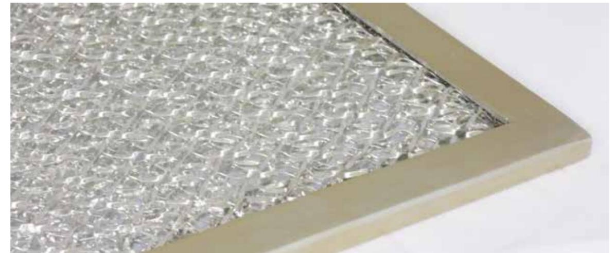
Aluminum screen EMC & dust filter ventilation panels consist of multi-layer expanded aluminum foil mesh trapped in a rigid extruded aluminum mounting frame, the frame can be supplied in a choice of sizes and profiles. Panels can be treated with a variety of finishes to provide corrosion protection. Air filter oil can be applied to the aluminum filter media to assist in dirt and dust retention.
