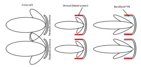
**Example 2** – To suppress noise reflected by casing.
