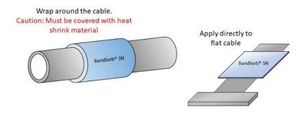
**Example 3** – To suppress radiation noises from LSI and IC.
